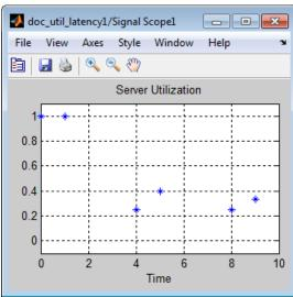
In a longer simulation, the differences in the value of  ${\bf util}$  compared to its theoretical definition become less pronounced.
